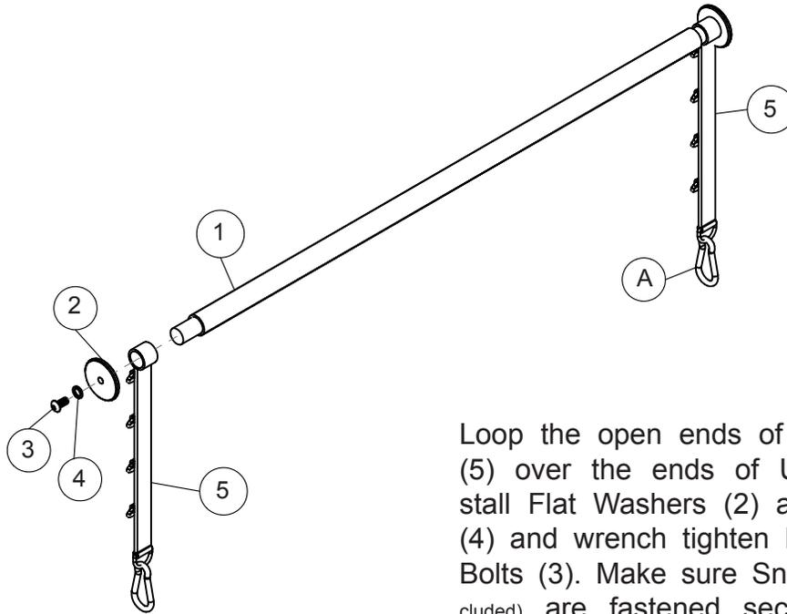
Loop the open ends of Utility Bar Straps (5) over the ends of Utility Bar (1). Install Flat Washers (2) and Lock Washers (4) and wrench tighten Round Allen Head Bolts (3). Make sure Snap Links (A) (not included) are fastened securely before use.
